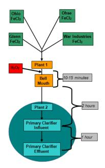
Figure 1. Schematic of Plant 1 to Plant 2 Chemical Odor Control
