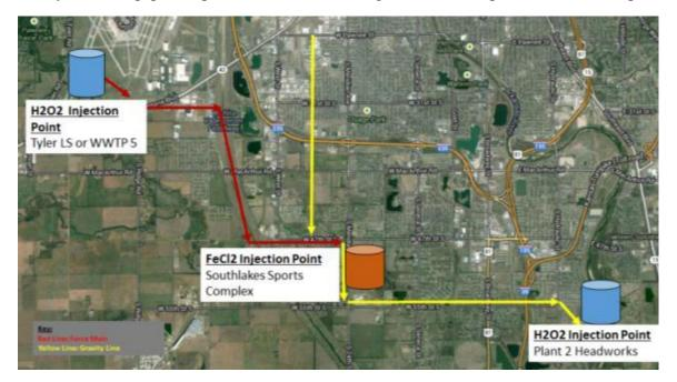
Figure 3. Plant 2 Collection System Proposed Chemical Dosing Sites
