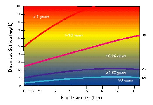
Figure 4. Effect of H<sub>2</sub>S on Concrete Pipe (American Concrete Pipe Association)
