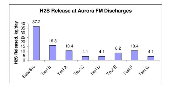
Figure 2. Gaseous H<sub>2</sub>S Released at Turbulent Aurora Forcemain Discharges
