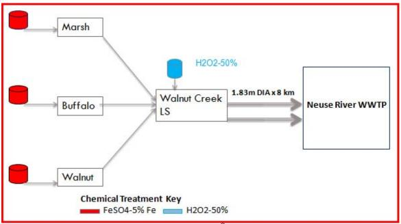
**Figure 3. Simplified Collection System PRI-SC<sup>®</sup> Schematic**
