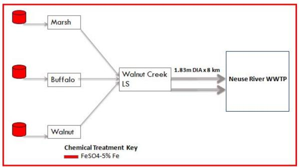
Figure 2. Simplified Collection System Schematic with FeSO4 Feed Sites
