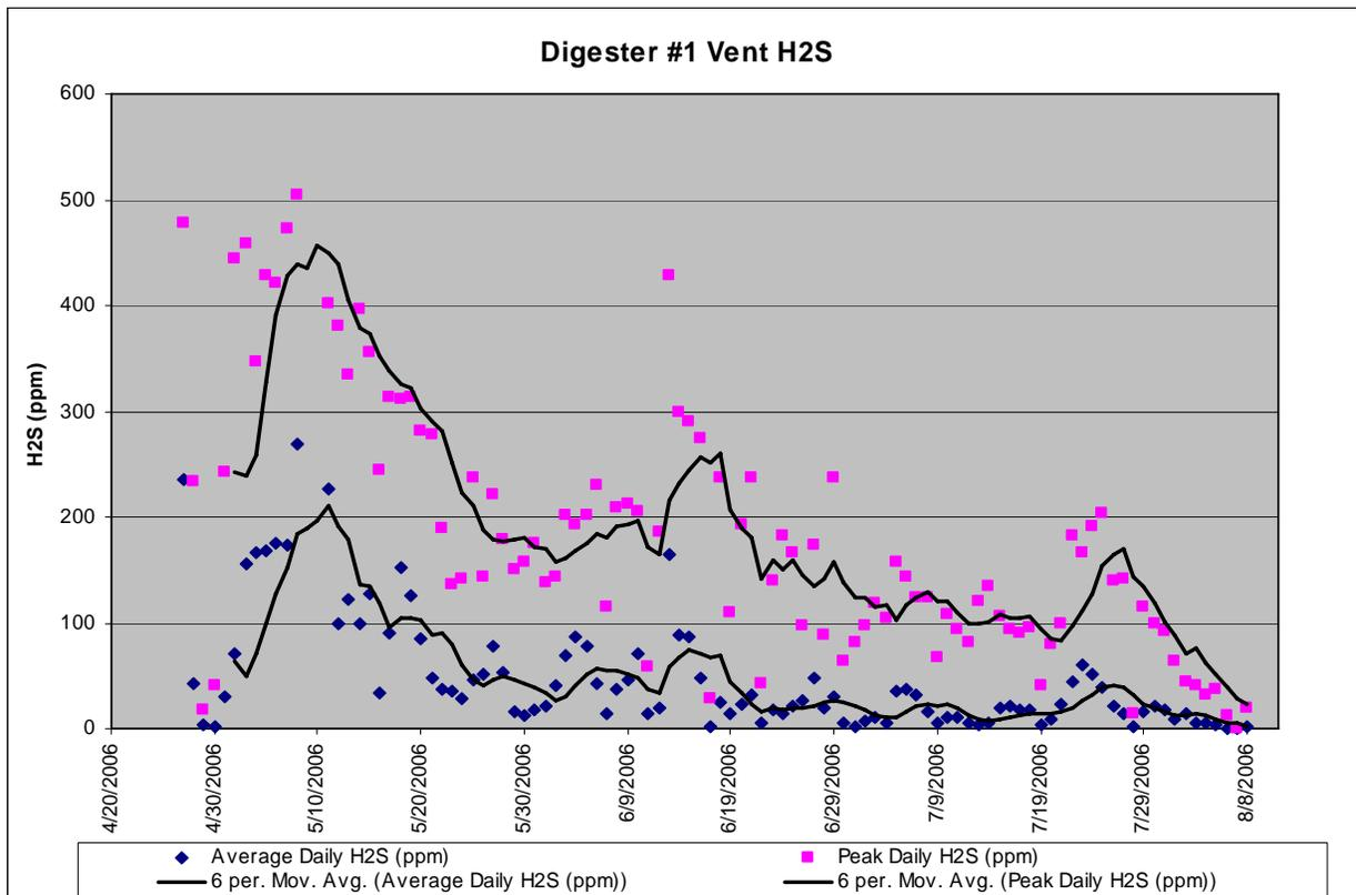
**Figure 8: Daily average and maximum hydrogen sulfide levels at the vent of the secondary digester. Recorded H<sub>2</sub>S levels were susceptible to interference from wind conditions.**
