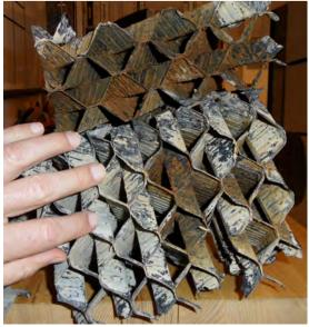
Figure 22. Close up from end view showing open passages and fill texture
