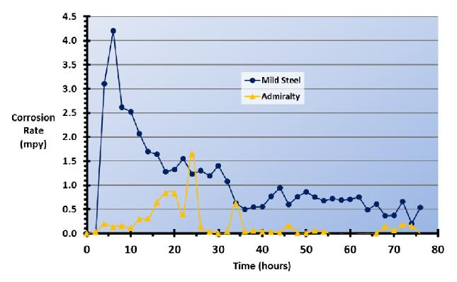
Figure 41. On-line corrosion rate measurements for mild steel and admiralty brass during the first peroxide cleaning procedure. Corrosion rates increased for several hours after the initial shot feed and returned to baseline within 36 hours.
