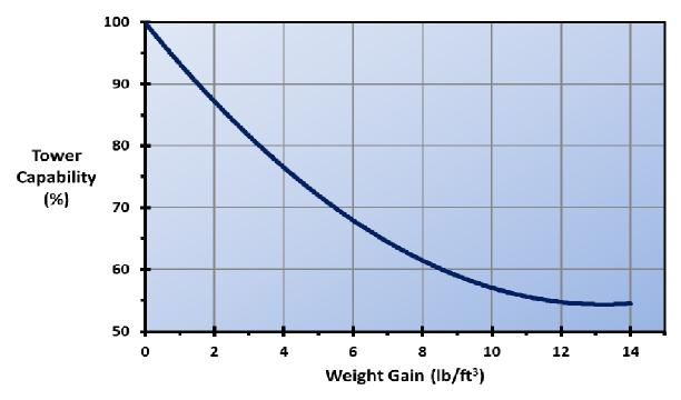
Figure 7. Tower capability loss vs. fill weight gain for a standard offset flute cellular plastic fill pack.<sup>5</sup>
