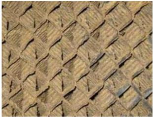
Figure 29. Cross-fluted tower fill fouled with a slime-clay matrix prior to peroxide cleaning
