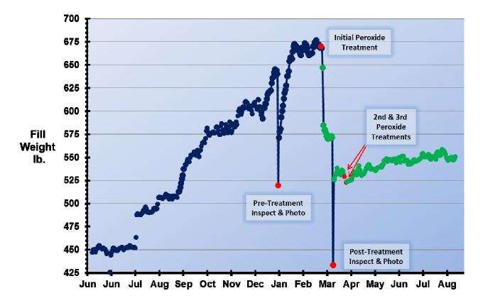
Figure 37. On-line fill pack weight measurements from installation through peroxide cleaning. The initial peroxide cleaning removed 150 lb. of deposit weight from the test cell.
