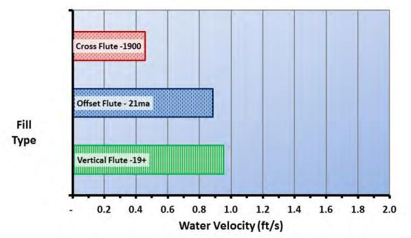
Figure 4. Water film velocity for typical cellular plastic fill packs of cross-fluted and fouling resistant designs.<sup>3</sup>
