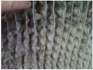
Figure 10. Fouled cross-flow, external louver high efficiency fill pack
