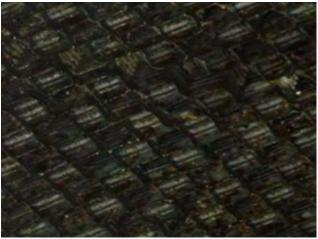
Figure 30. Cross-fluted tower fill after peroxide cleaning.
