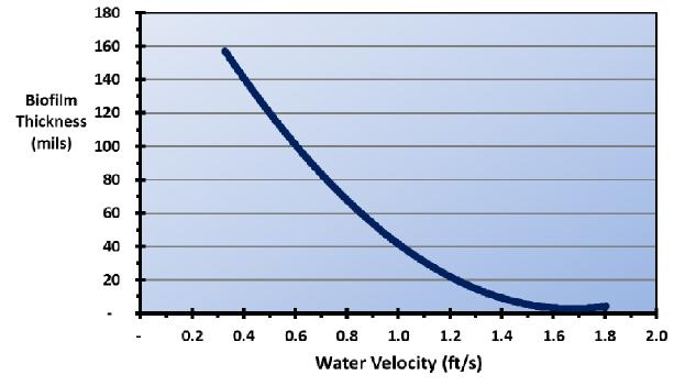
Figure 3. Biofilm thickness as a function of water velocity<sup>2</sup>
