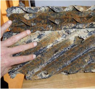
Figure 21. Close up of cross-fluted fill 7 months after restoring proper treatment
