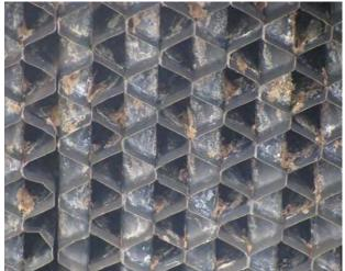
Figure 26. Close-up of underside of fill after peroxide cleaning showing biofouling substantially removed.
