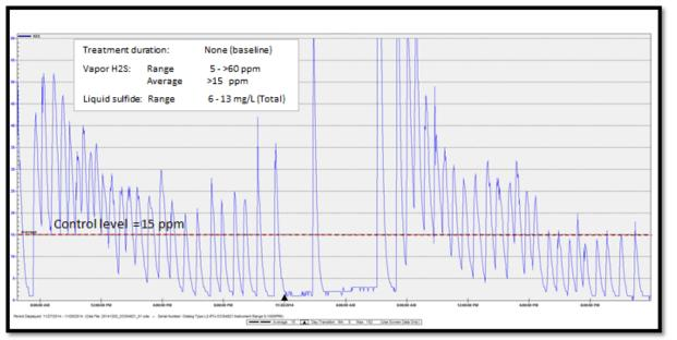
Figure 7 shows the  $H_2S$  readings through the first 13 days following the initial 24-hr Cloevis treatment. The results show a 3-4 day period where  $H_2S$  production is completely suppressed, followed by a slow recovery to where  $H_2S$  control levels began to be exceeded on Day-8.
